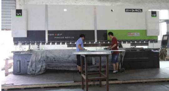
折弯成形机 (华南最大: 7000mm) Bending and Forming Machine (It is the largest in South China: 7000mm)
